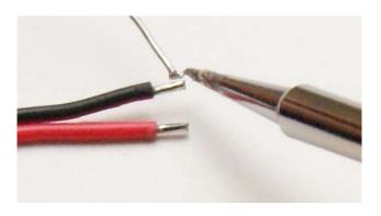
When soldering power wires to LED tape, prepare the wire by first "tinning" the stripped ends of each wire lead. Place the tip of the hot soldering iron against the wire and apply a light, even coat of solder as shown.
