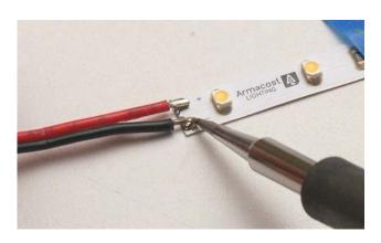
Once the wire leads and copper pads are tinned, simply join the wires to the copper pads and solder using a clean soldering tip. No extra solder is required since tinning has been done. Be sure to maintain correct + / - polarity.
