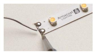
The same basic tinning process is also required on each of the copper pads on the LED tape lighting. Be sure to use painter's masking tape to secure the LED tape when you are soldering.
