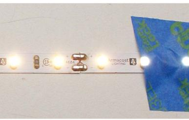
Be sure to power up your LED lighting prior to final installation. Check to ensure that all tape sections are lighting properly and connections are solid.
