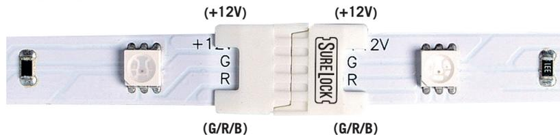
If the +12V/G/R/B marks do not line up, flip the tape strip and use the opposite end for proper +12V/G/R/B alignment.
