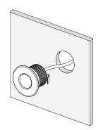
Wall surface should be a minimum of 3/8 in. thick when light is mounted with spring clip. For thinner walls, use Armacost Lighting's screw-on backing nut, (Item # 950000), sold separately.
